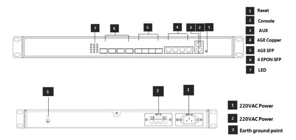
Wodaplug WDS1U4PGE EPON has 4 EPON SFP ports, 4GE(copper) and 4SFP slots Combo interface for uplink, 1 console port and 1 GE network management port.
